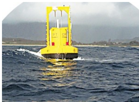
Wave energy generating “PowerBuoy” – Kaneohe Bay FOUO
